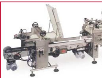
New sanitary frame and angle panning section for none twist loaf.
